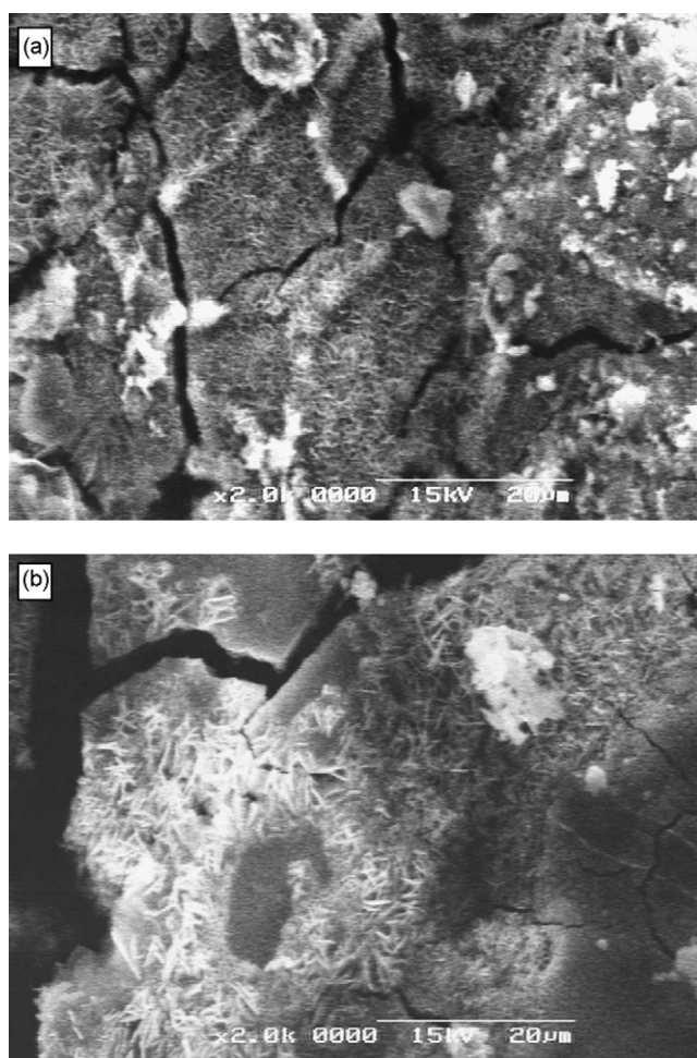
Fig. 6. Surface morphology for cast iron scraps after corrosion. (a) B=0 mT and (b) B=15 mT.
